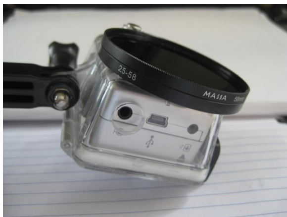
Figure 12 Final product with hole drilled for external microphone
