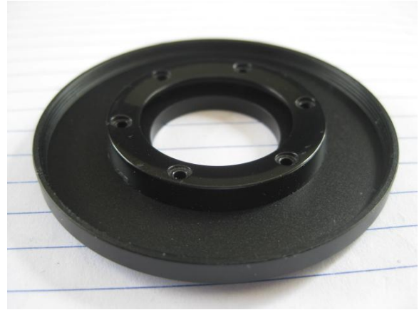
Figure 6. Lens retainer as drill template
