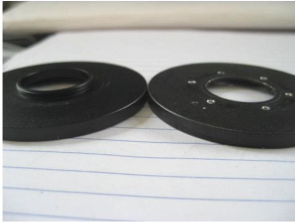
Figure 4. Filter adapter, before and after filing off the flange, and transferring screw holes.
