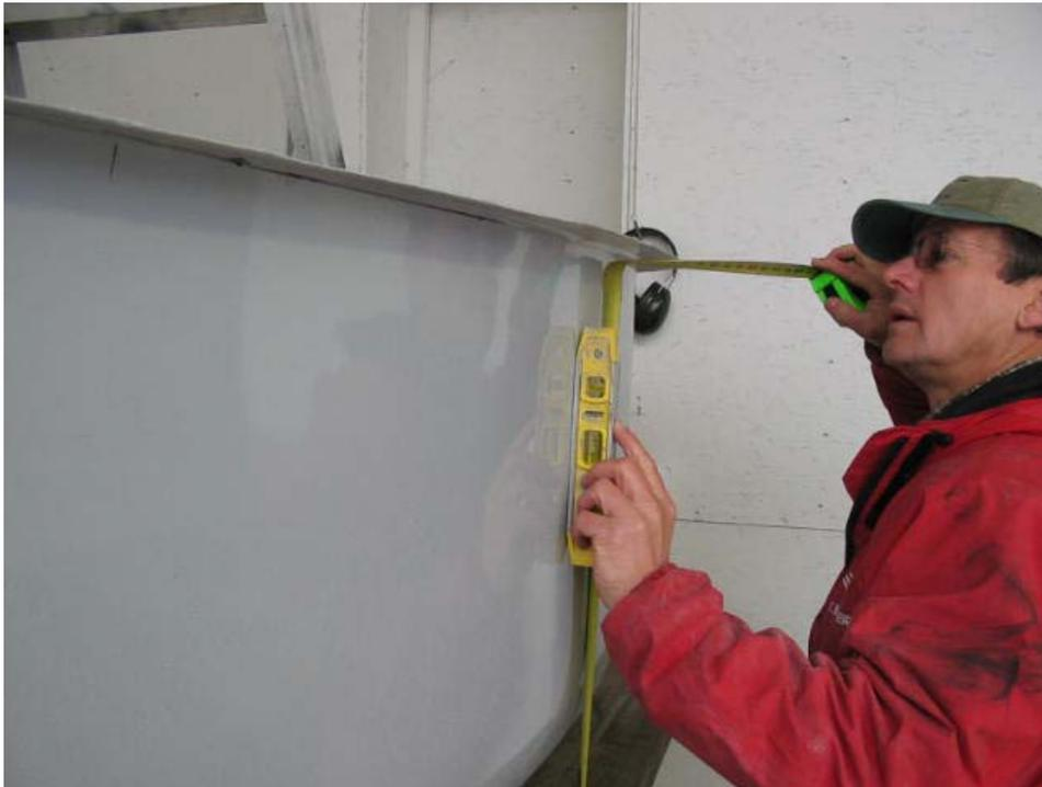
3/ Using measurements from the old tip if retrofitting, or pushing the tip onto the wing, mark roughly where the cut out for the aileron spade will be (bottom surface only). Leave  $\frac{1}{2}$ " excess material.
