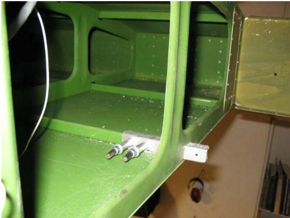
9/ Attach spar extension to angles, drill and cleco.
