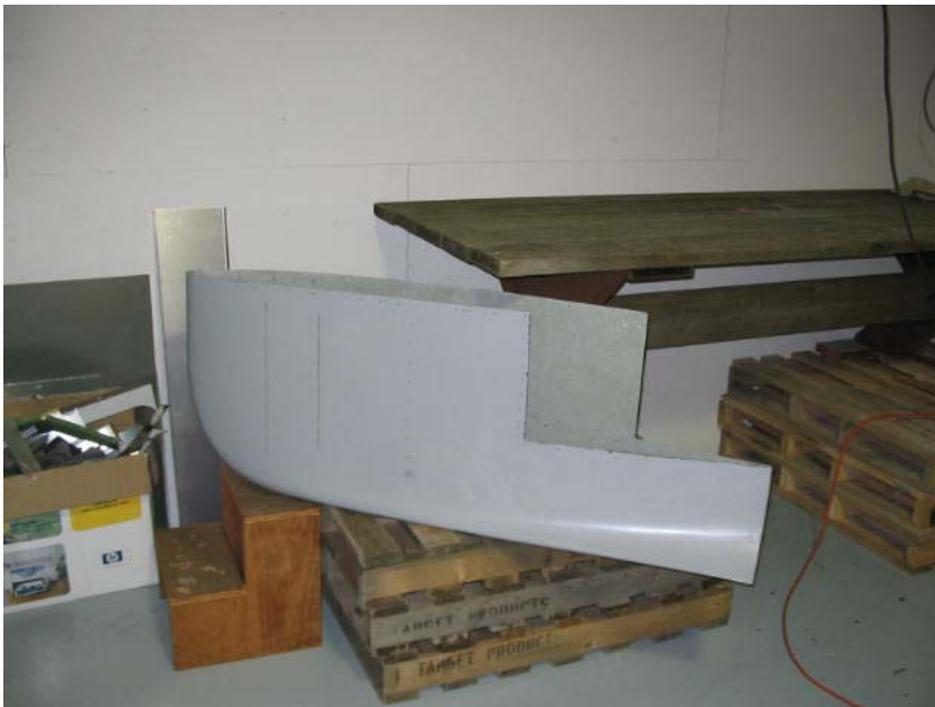
4/ Push tip onto wing and position carefully. Transfer stringer rivet lines and main spar rivet lines from wing to tip.
